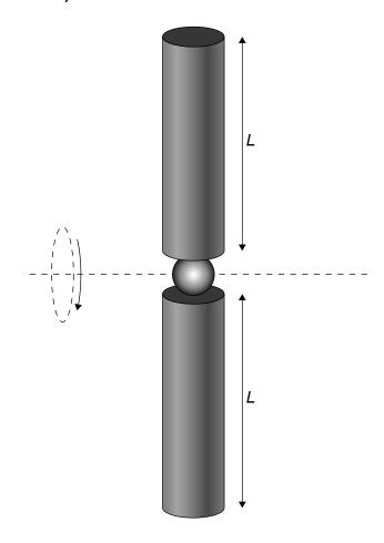
(b) A two-blade propeller can be modelled using the two-cylinder arrangement in (a)(iii).
